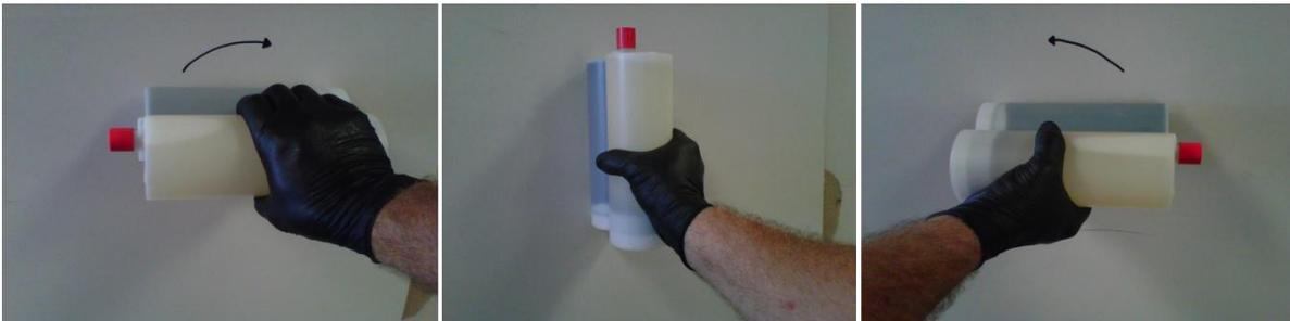
To keep from cross contaminating the chemicals, keep the cartridge pointed up once the cap is removed, until you are ready to pull the trigger.
