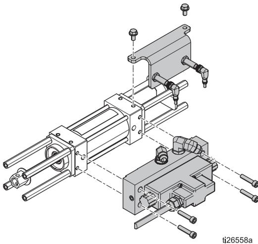
4. Follow **Pumpline Disassembly**, page 9. Then remove the hydraulic cylinder from the proportioner.
