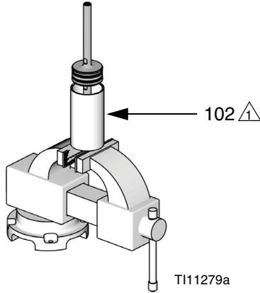
⚠ Apply lithium grease to the inside of each end of the cylinder.
