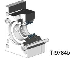
5. Insert piston rod (28) through throat seal (29) on front of block. Use grease to aid with insertion if needed.
