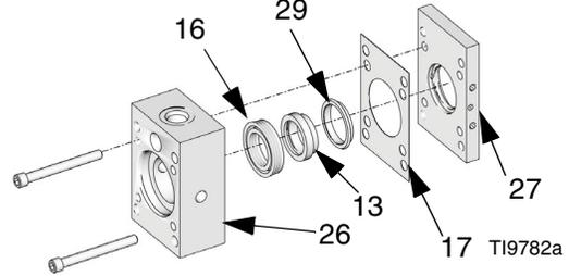
4. Ensure plate is parallel with block. Carefully tighten screws until plate is flush with block. Be sure to press seal straight into bore.
