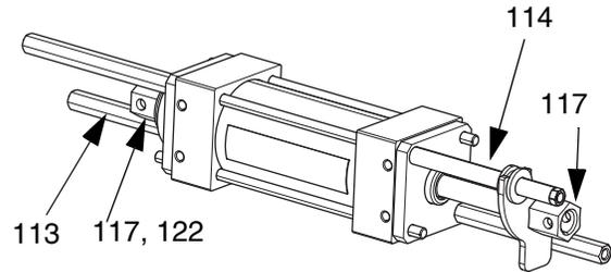
**NOTE:** The clevises (117) and the baffle jam nut (122) were installed with high strength thread sealant. The following steps will require significant force to break loose the baffle jam nut and clevises.
