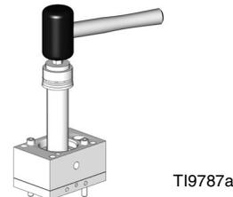
6. Place assembly in a vise, and tap piston rod (28) through throat seal (29) and bearing.
