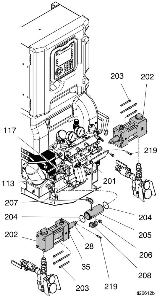
2. Install elbow fittings (207, 208) into lube cylinder (205) and install lube cylinder over left clevis (117). Ensure clevis pin hole in lube cylinder is horizontal, in line with the hole in the left clevis.
