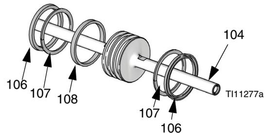
**Insert Piston into Cylinder**
