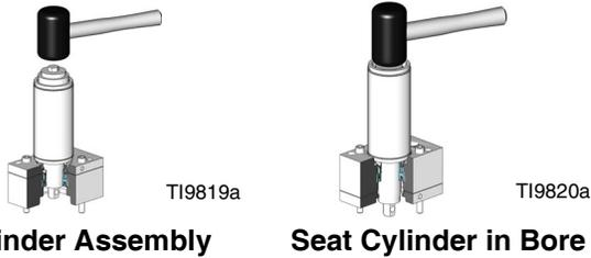
9. Lubricate and assemble o-rings (2) to crossover tube (24). Insert crossover tube into outlet flange (26). Softly tap crossover tube into bore until it seats.
