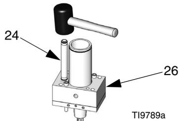
10. Carefully align cylinder (12) and crossover tube (24) to bores in pump base (23). Tap pump base until the cylinder is fully seated in bore.
