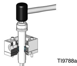
7. Lubricate and assemble o-rings (1) to cylinder (12).
