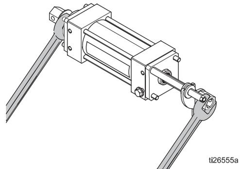
**If the left clevis and baffle jam nut break loose from the hydraulic piston shaft:**
