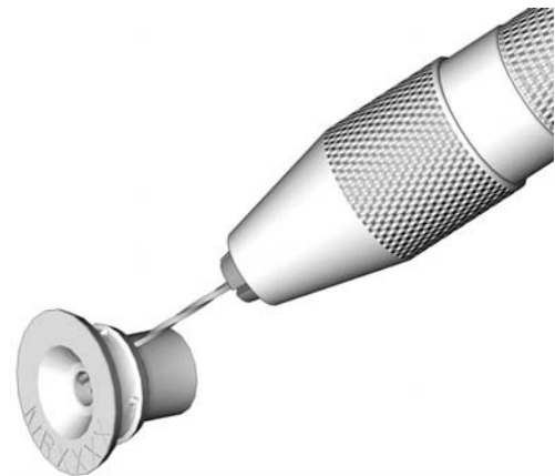
FIG. 2. Cleaning Component B (Resin) Ports
