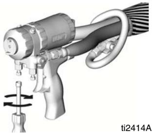
17. Disengage gun piston safety lock.
