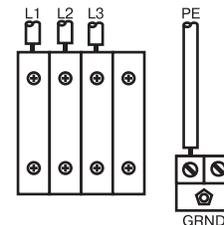
**380V, 3 Phase WYE:** Use a screwdriver to connect four power leads to the top terminals as shown. Connect neutral only to N. Connect green to ground (GND). See page 17 for proper jumper positions.
