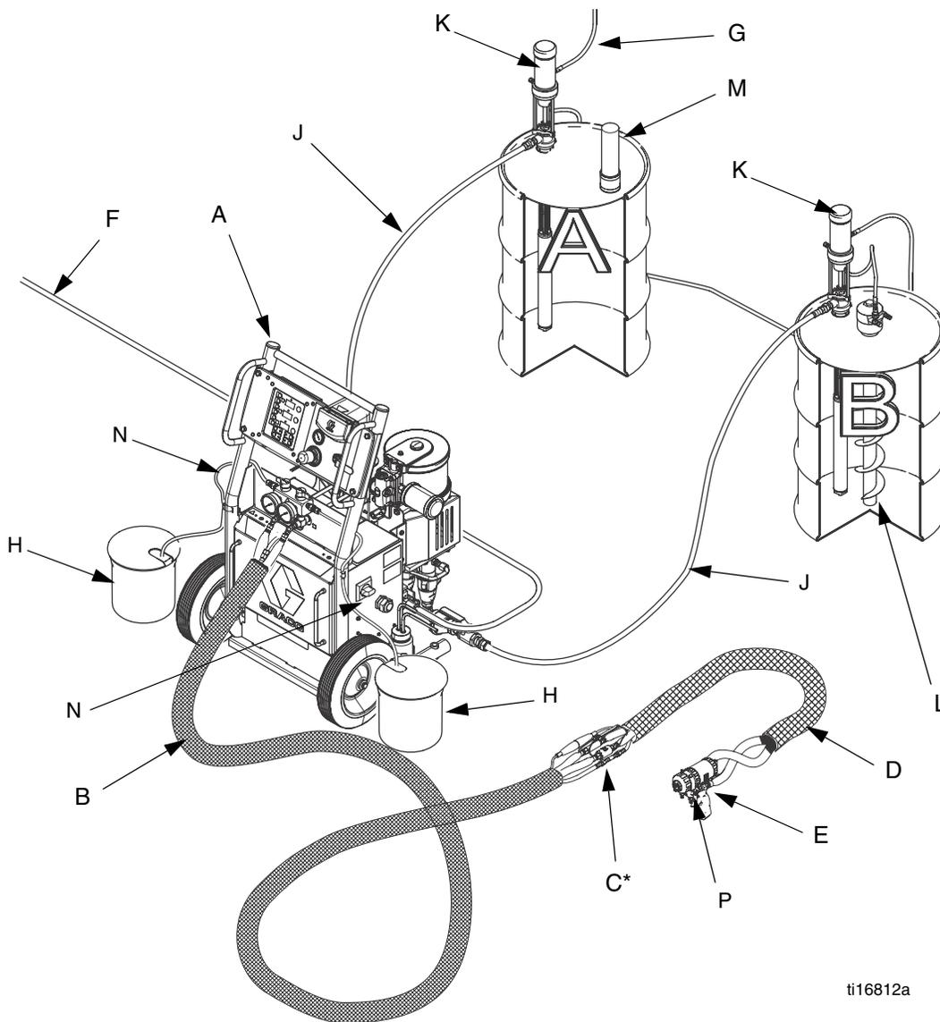
\* Shown exposed for clarity. Wrap with tape during operation.
