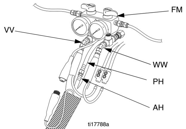
**NOTE:** Manifold hose fittings (VV, WW) allow use of 1/4 in. and 3/8 in. ID Reactor heated fluid hoses.
